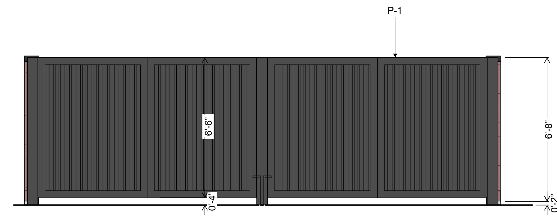
DUMPSTER ENCLOSURE - FRONT ELEVATION SCALE: 3/8" = 1'-0"
